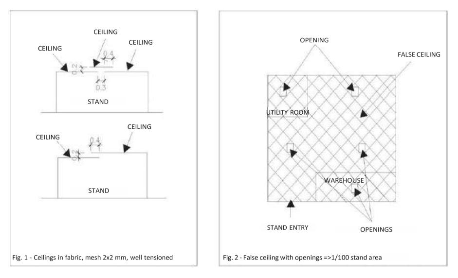
3 - False ceilings can be made of a wide mesh fabric (max. 2x2 mm), well tensioned. Thick mesh fabrics fall within the scope of point 2.
